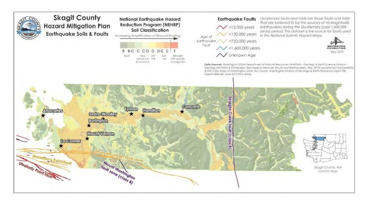
Figure 6-4 Skagit County NEHRP Soils Classifications and Local Area Faults
