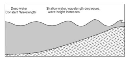
Figure 10-2 Change in Wave Behavior with Reduced Water Depth
