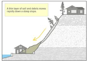
Figure 8-2 Shallow Colluvial Slide
