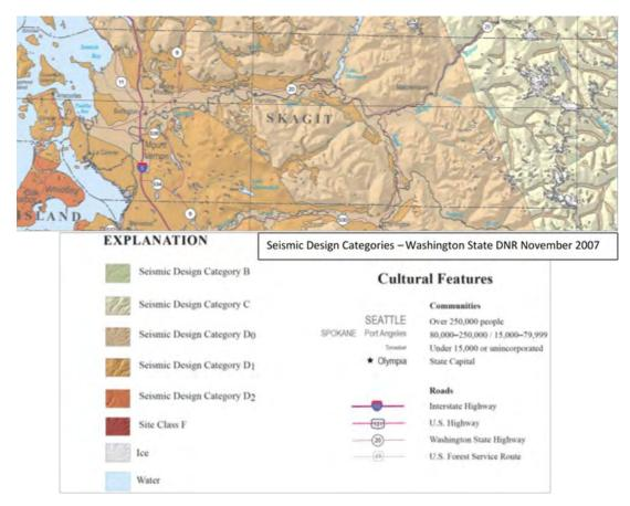
Figure 6-3 Skagit County Seismic Design Codes
